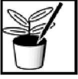
An icon showing a plant in a pot with a probe inserted into the soil.     | Insert the probe at least 50 mm deep into the soil or hold it in the solution or in air.                                                                                                                        |
