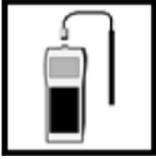
An icon showing a probe with a cable being inserted into an 8-pin socket. | Connect the probe to the 8-pin socket.<br>If the pH function module is also installed, its probe can be connected to the BNC socket at the same time. The display shows then a pH value compensated to 25°C.    |
