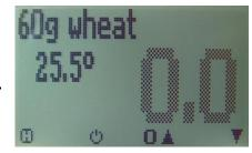
6. Fill up the cup with the sample material (+/- 0.5g). The filling quantity needed is shown on the upper left corner on the display of the device.
