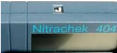
Sliding switch to switch off the beeper
